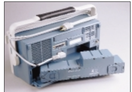
TDS 3BAT – Battery Pack being installed.
